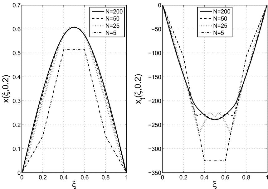
**Fig. 6** 1. Vertical displacement at  $t = 0.2$  for different numbers of nodes in the distributed control problem (*left*). 2. Vertical velocity at  $t = 0.2$  for different numbers of nodes in the distributed control problem (*right*)
