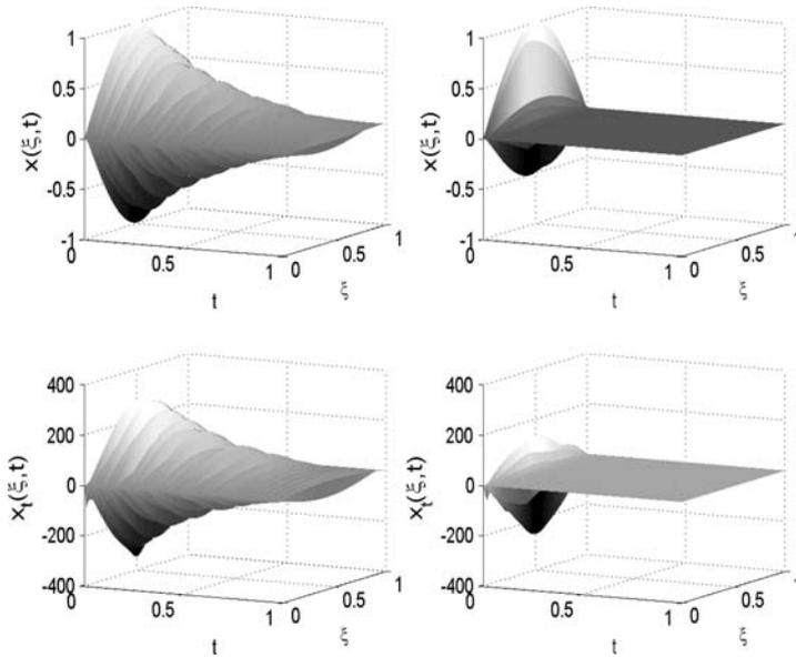
**Fig. 1** 1. Uncontrolled vertical displacement (*up-left*). 2. Controlled vertical displacement with point control at  $\xi = 0.4$  (*up-right*). 3. Uncontrolled vertical velocity (*down-left*). 4. Controlled vertical velocity with point control at  $\xi = 0.4$  (*down-right*)
