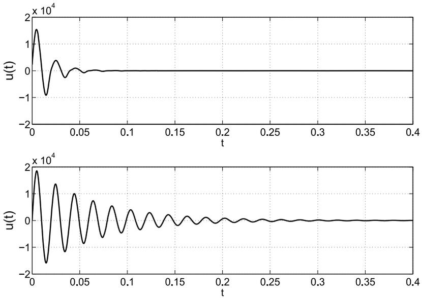
**Fig. 3** 1. Control signal for the point problem (*up*). 2. Control signal for the distributed problem (*down*)
