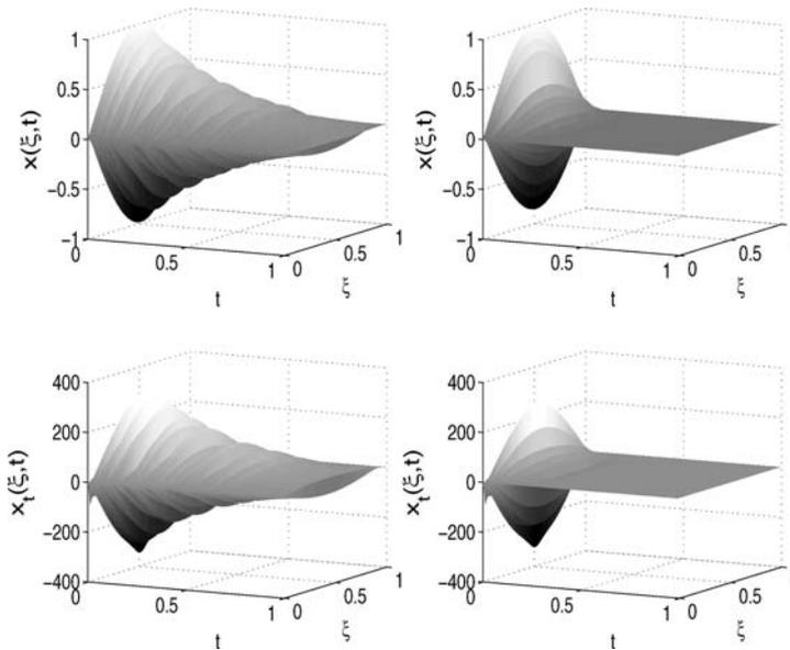
**Fig. 2** 1. Uncontrolled vertical displacement (*up-left*). 2. Controlled vertical displacement with distributed control along  $I_c = [0.4, 0.6]$  (*up-right*). 3. Uncontrolled vertical velocity (*down-left*). 4. Controlled vertical velocity with distributed control along  $I_c = [0.4, 0.6]$  (*down-right*)
