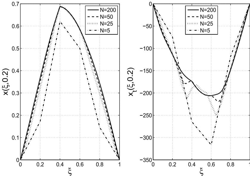
**Fig. 4** 1. Vertical displacement at  $t = 0.2$  for different numbers of nodes in the point control problem (*left*). 2. Vertical velocity at  $t = 0.2$  for different numbers of nodes in the point control problem (*right*)
